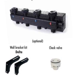
Two-chamber steel manifold **C 60 DN 25** - 2, 3 or 4 heating circuits was created to simplify installation of pump groups. The factory manifold is equipped with EPP insulation. In addition, the manifold has an output DN 20 on the return side for connecting pressure vessel and the output DN 25 on the power supply for connecting the safety group. On request, the manifold can be equipped with a set of mounting brackets on the wall **DELTA** (see bushings M8).
